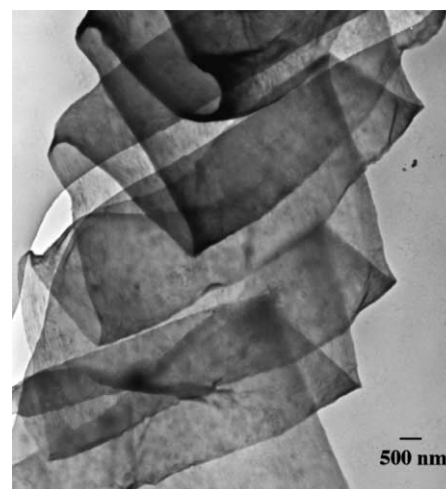
Fig. 2. Bright field TEM image of a ribbon shaped nanofiber.
